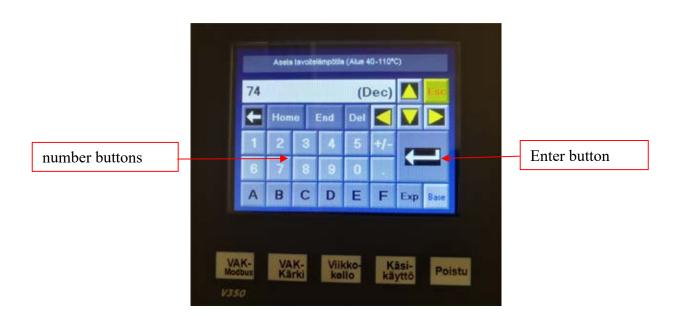
After confirmation of the temperature value, the display returns to the previous screen. Press "Poistu" (exit) to return to the home screen.
