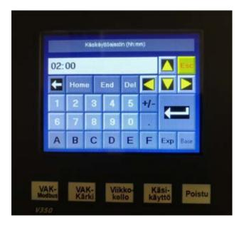
Use the number buttons to choose the desired time (hh:mm) and the Enter button to confirm. The ON time can be set between 1 and 12 hours.
