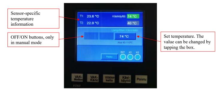
The setting can be changed by tapping the set temperature box. The temperature can be adjusted between 40 and 110°C. The desired temperature is entered using the number buttons and confirmed by pressing the Enter button.
