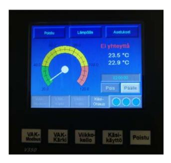
If manual control has been selected as the operating mode, "Käsiohjaus" (manual control) is highlighted at the bottom of the screen and "Pois"/"Päälle" (Off/On) buttons are displayed on the screen. The ON time is displayed above the Off/On buttons.
