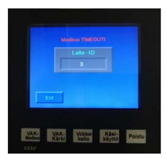
Modbus control-related specification of the device ID.
